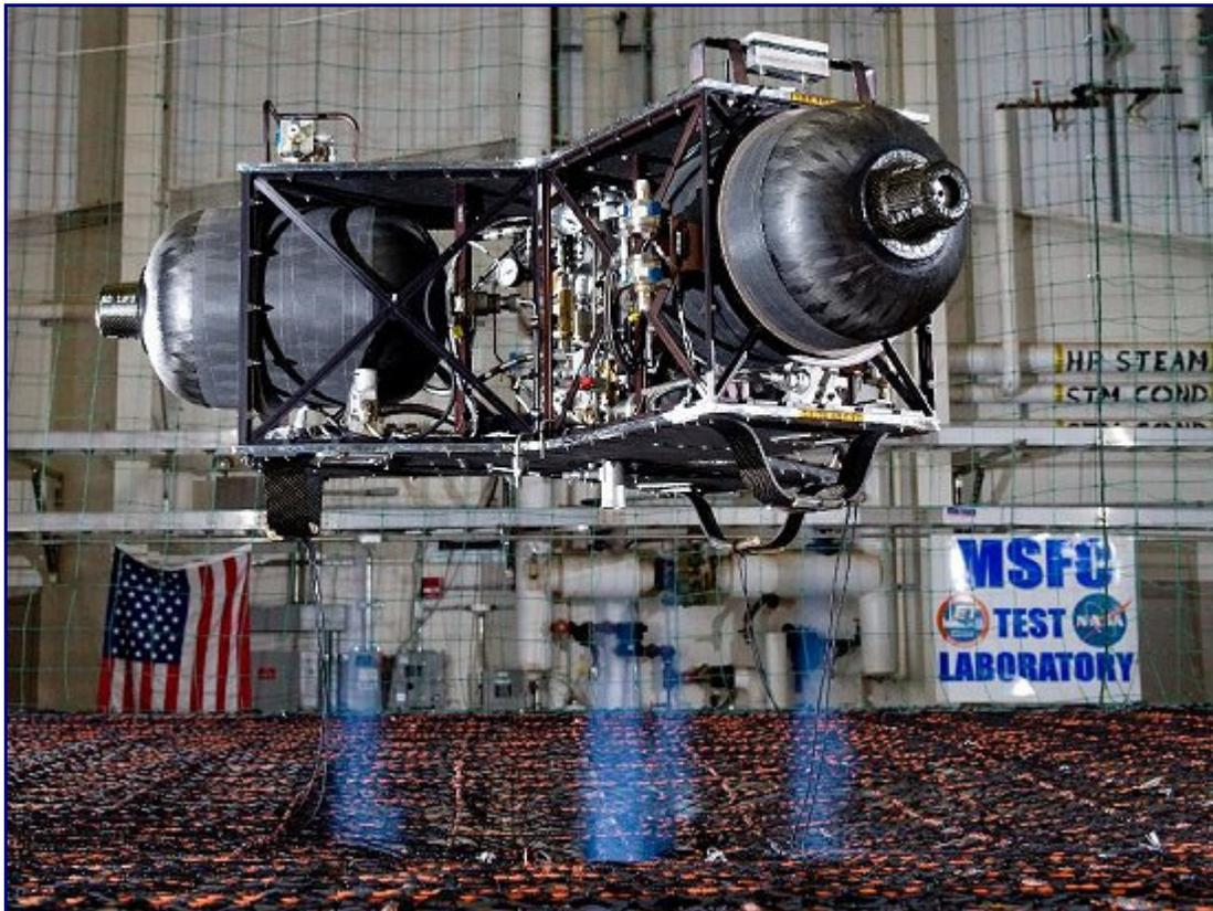
"What we've got here is a 'flying testbed' to help us to learn how to hover<sup>1</sup> and land on the Moon," says Mulac. He's conducting the tests in collaboration with other engineers from NASA, the John Hopkins University Applied Physics Laboratory, and the Von Braun Center for Science and Innovation.
