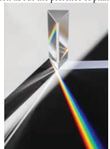
Prism is a common disperser
